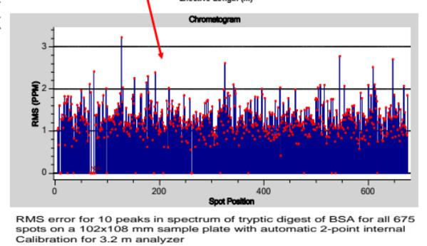
RMS error for 10 peaks in spectrum of tryptic digest of BSA for all 675 spots on a 102x108 mm sample plate with automatic 2-point internal Calibration for 3.2 m analyzer
